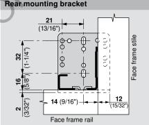
**NOTE:** For frame applications Minimum three screws per bracket
