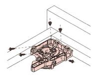
3. Lay the drawer bottom onto the slide then push the drawer into the cabinet.
