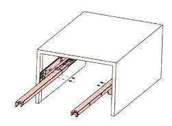
4. For removal, hold the handle and pull out the drawer.
